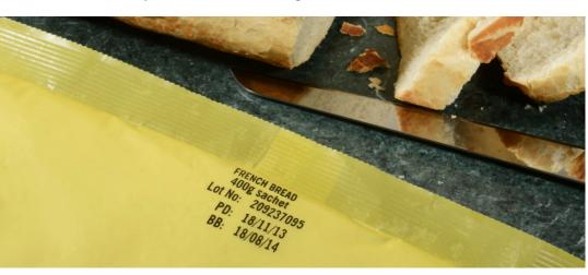
date packed and best before date onto plastic sachets at speeds up to 50 packs per minute.
